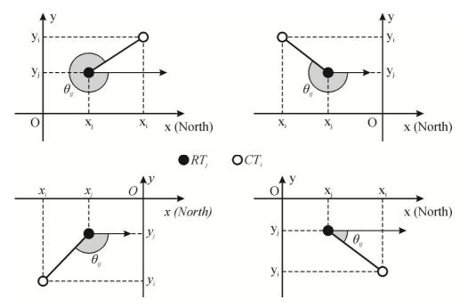
Figure 2. Possible situations between a CT, it's corresponding RT and their azimuths
