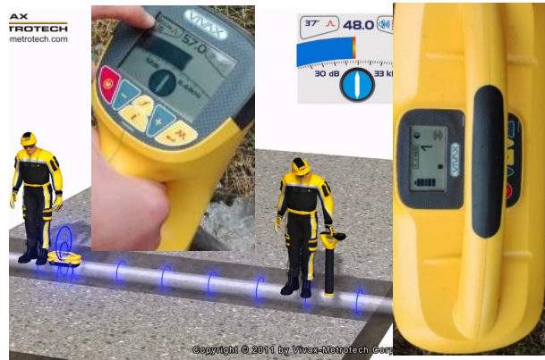
Figure 5. vLocPro receiver (middle), transmitter (right) and principle of operation.
