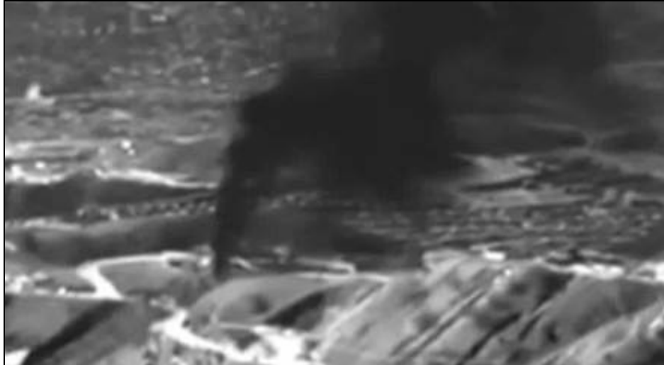
Figure 2. Example of a thermal image of a cloud of hydrocarbons (www.cnn.com).
